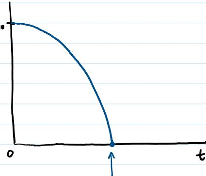
$$t_{\text{floor}} = \frac{C_1}{g} + \sqrt{\frac{2C_2 g + C_1^2}{g}} \quad \text{for } 0 = \frac{g}{2} t^2 + C_1 t + C_2$$
